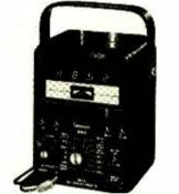
of continuous operation. Recharging is automatic when the line cord is plugged in and the function selector is in the BATT CHRG ONLY position. A LED on the panel shows when the battery is being charged.
