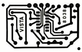
FIG.4—FULL-SIZE FOIL PATTERN of the circuit board for the generator.
