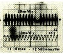
FIG. 9—CHROMA IC AMPLIFIER OUTPUT and subcarrier sinewave.
