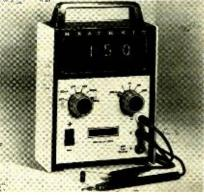
est ranges is 10 mV, 10  $\mu$ A and 1 ohm. Accuracy (full scale  $\pm 1$  digit): dc volts  $\pm 1\%$ ; dc and ac current and ac volts  $\pm 1.5\%$ ; ohms  $\pm 2\%$ .
