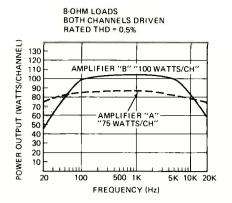
FIG. 2---"LOWER POWERED" AMPLIFIER A can actually produce more power at frequencies in shaded areas because of its better power bandwidth.
