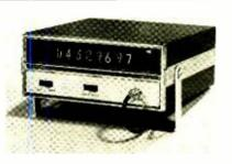
FIG. 6—THIS FREQUENCY COUNTER has eight digits in its readout and goes out to 120 MHz.
