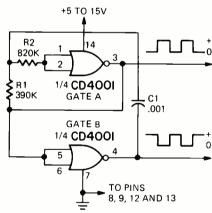
FIG. 29—COMPENSATED 1-KHZ astable multivibrator.
