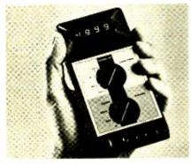
Voltage ranges are 2, 20, 200, and 1000 volts dc and peak ac with 1-mV resolution. Resistance ranges are 2K, 20K, 200K and 2 megohms. Capacitance is read in four ranges from 2 to 2000 nF (.002 to 2.0  $\mu$ F) with resolutions of 1, 10, 100 and 1000 pF.
