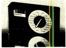
Voltage ranges (ac and dc) are 2, 20, 200 and 1 kV with 1 mV resolution. Input impedance is 10 megohins on dc and 2 megs shunted by 40 pF on ac. Accuracy is  $\pm 0.5\%$  of reading +.05%of range on 2-volt dc range; ±:0 75% of reading +.05% of range on the remaining dc ranges.
