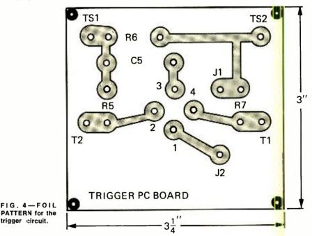
toggle or rocker switch instead of the jumper between points J1 and J2 in Fig. 3. For a choice of 50, 100, 150 or 200 watt-seconds, modify the circuit board by removing the copper foil paths between the positive terminals of C3 and C5 and C4 and C6. Install a heavy-duty single-pole, 4-position *progressive-shorting* switch on the housing top. Connect the four terminals to the positive terminals on C3— C6 and the arm to point T2.
