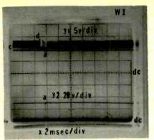
FIG. 2—COMPOSITE VIDEO and sync wave-
