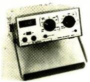
Accuracy is  $\pm 0.2\%$  of reading +1 digit on 1000 mV dc,  $\pm 0.5\%$  of reading +1 digit on 10, 100, 1000 Vdc and the five current ranges;  $\pm 1\%$  of reading +2 digits on acV;  $\pm 1.5\%$  of reading +2 digits on ac current and  $\pm 1\%$  of reading +1 digit on all resistance ranges.
