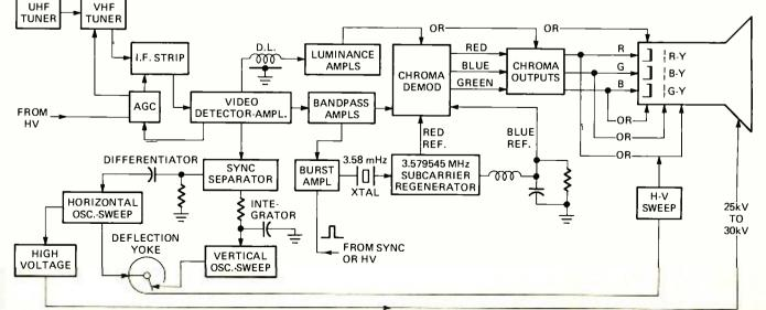
FIG. 1-BLOCK DIAGRAM OF TYPICAL COLOR TV is the same for tube, transistor or IC circuits.
