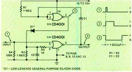
FIG. 24—IMPROVED COMPENSATED monostable multivibrator.
