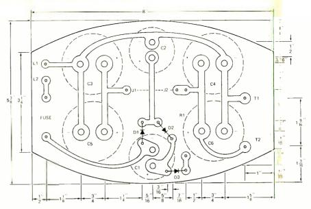
FIG. 3--FOIL PATTERN for parallel capacitor bank which provides 200 watt-seccnc output (connect jumper between J1 and J2). With modifications, the foil pattern is also used for the multiple power output flash (see text).
