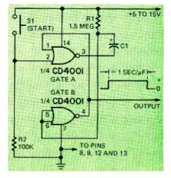
FIG. 22—"NOISELESS" PUSH BUTTON or manually-triggered monostable.
