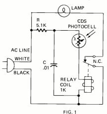
cell (abbreviated CdS), then through the coil of the relay. The CdS cell here is used as a variable resistor. The arrows are the symbol for a lightactuated device.
