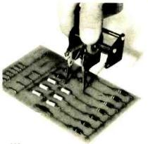
leads against sides of pointers with thumb and forefinger. All axial lead components are accommodated, e.g., resistors, capacitors, diodes, transistors, inductors, etc. up to 1/2 in. diameter x 11/2 in. long with maximum distance between inside of bends of 1.725 in. \$32.50-complete with spare set of lead guides .- Harwil Co., 903 Colorado Avenue, Santa Monica, CA 90401.
