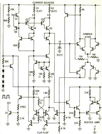
FIG. 2—DETAILED CIRCUIT DIAGRAM of the Intersil 8038 IC waveform generator.
