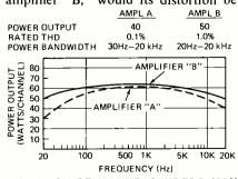
FIG. 3—SINCE MANUFACTURERS MAY QUOTE different rated harmonic distortions for their products, a fair comparison of these two amplifiers cannot be made without further information or lab testing.
