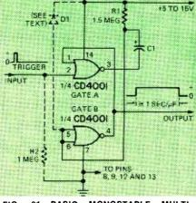
FIG. 21—BASIC MONOSTABLE MULTI-VIBRATOR or pulse stretcher.
