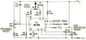
FIG. 3—SCHEMATIC OF THE GENERATOR. Circuit is built around the Intersil 8038 waveform generator IC.
