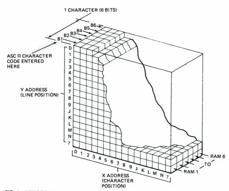
FIG. 2—MEMORY FORMAT. The 6-bit character is entered into memory in ASC11 code. The memory location is selected in accordance with the respective position on the page (line and character position.)
