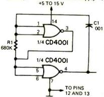
FIG. 30-BUFFERED-OUTPUT 1-KHZ astable
