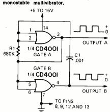
FIG. 26—BASIC 1-KHZ ASTABLE multivibrator or square-wave generator.
