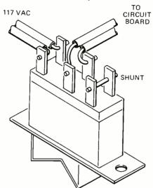
FIG. 5-AC POWER SWITCH wiring.
