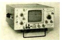
modes and stable, high-speed gated trigger capable of locking any signal from dc to 40 MHz, including TV line and frame. Special operating requirement such as dc trigger or  $\times 5$  magnification is obtained by pressing the appropriate button. Also incorporates internal delay lines and offers optional battery pack. \$1,150.00—Scopes Unlimited, Inc., 1928 South Anaheim Blvd., Anaheim, CA 92805. *Circle 32 on reader service card*
